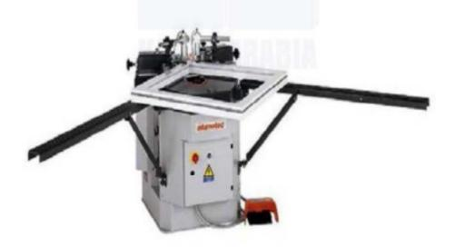
This machine is used for crimping of large dimensioned profiles to the highest quality standards. Easy adjustment and operation, short changeover times due to special blade changing system, special support head allows crimping of frames with in an inside dimension from 150mm.
