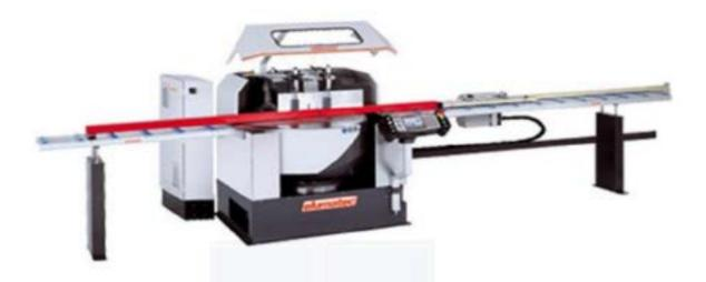
This machine also follows the principle of cutting from underneath. The patented saw arm suspension creates a cutting pressure towards the back fence which provides safe clamping of the workpiece. There is also free access for loading and unloading of profiles and automatically opens the safety of Hood.
